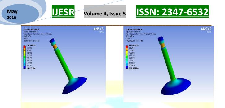
STRUCTURAL ANALYSIS POPPET VALVE WITH CARBON CARBON COMPOSITE MATERIAL MESH MODEL
